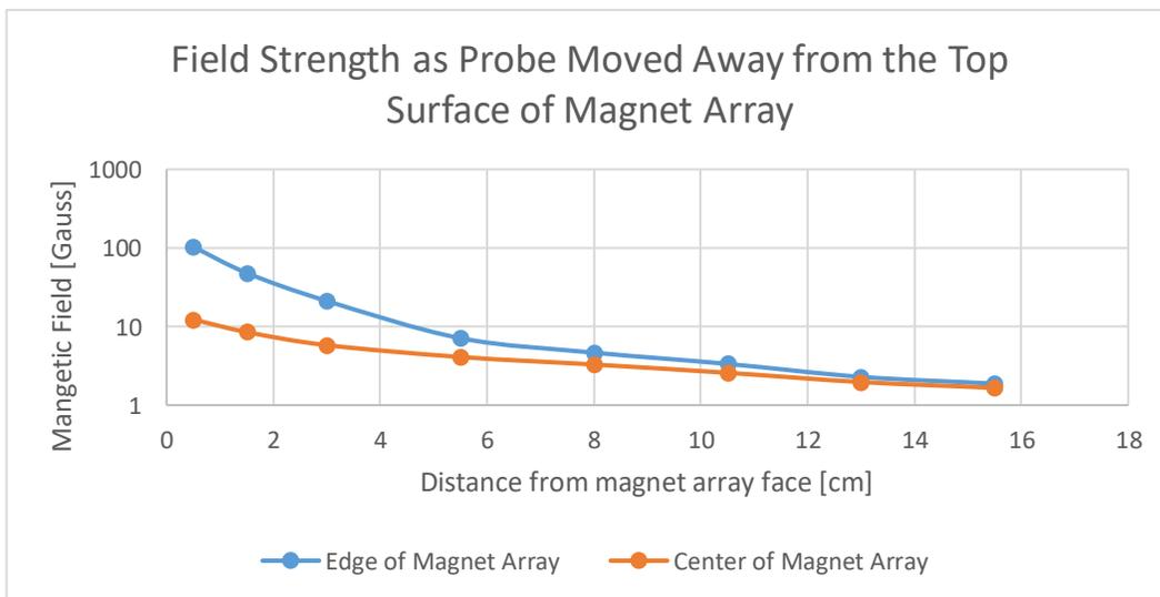
**Figure 5: Magnetic field magnitude above magnet array near the edge and center of the magnet array at different heights. Measurements were taken at a given Z, along the X-Axis, and Y = 0**
