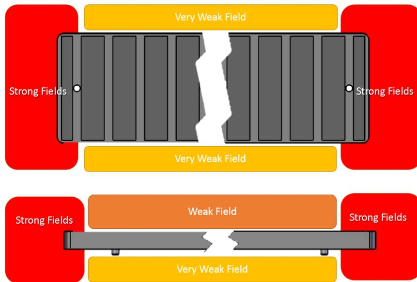
**Figure 1: Strength of the magnetic field magnitude for QS100 magnet array. Diagram for illustration purposes only.**
