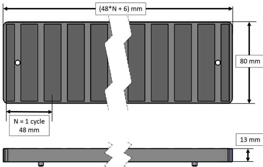
**Figure 3: Overall magnet array dimensions.**
