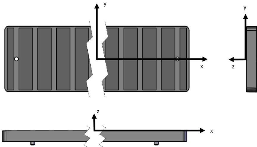
**Figure 2: Axis direction and location of origin with respect to the magnet array.**
