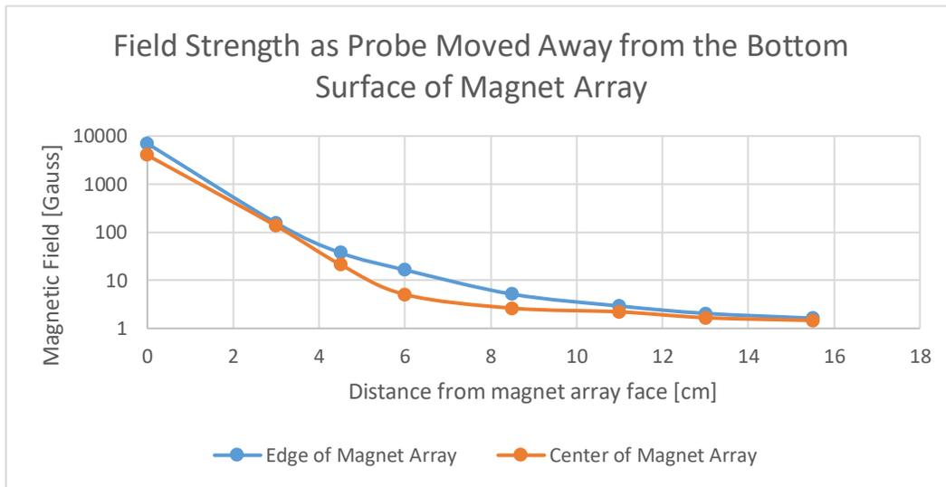
**Figure 4: Magnetic field magnitude below magnet array near the edge and center of the magnet array at different heights. Measurements were taken at a given Z, along the X-Axis, and Y = 0**
