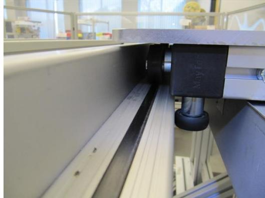
**Figure 3: A Wheel and Rail Guidance System**
