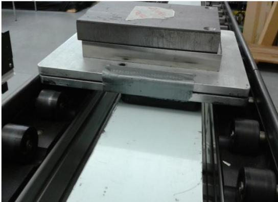
**Figure 2: A Roller Based Guidance System**
