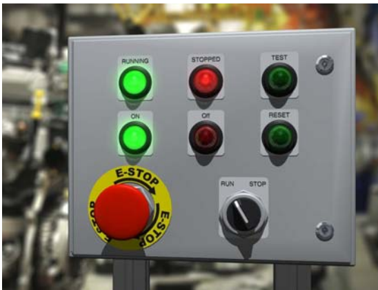
The "stopped" pilot light remains dimly illuminated even though the machine is currently running.
