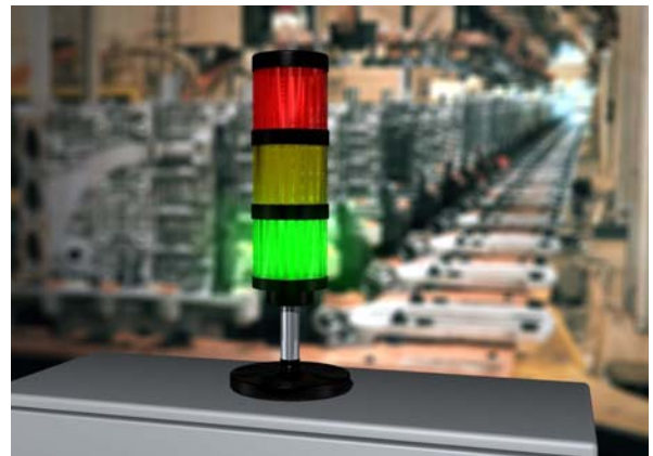
The red stack light LED, indicating the process is stopped, remains dimly illuminated even though the machine is currently running.
