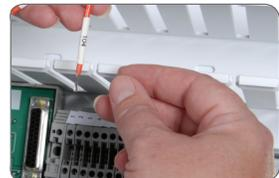
Assembler begins tagging each wire before connecting it to the terminal blocks.
