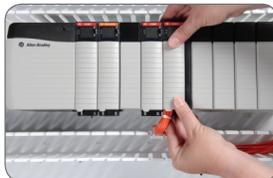
Finally half of the process is complete and PLC Module is wired and snapped into place.
