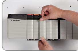
The assembler removes pre-wired 1492 cable from the box and connects the PLC end of the cable to the PLC.
