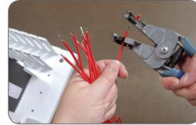
The assembler using the traditional method has measured and cut about 10 of the 18 wires needed for the same job. And there are numerous steps remaining.
