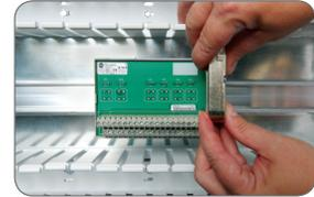
Then routes the cable through the wire duct and snaps the other end of the cable to the 1492 IFM Module.
