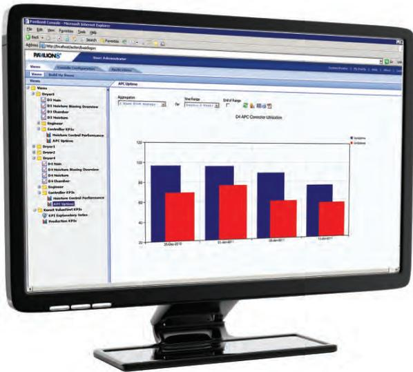
Specifically, the system utilizes Predictive Quality – Soft Sensors to provide in-line, inferential quality measurements and facilitates real-time and frequent control feedback. Rather than requiring an operator to manually check the drying process frequently, the system automatically collects data inputs every 15 seconds, resulting in a significant reduction of moisture content variation.
