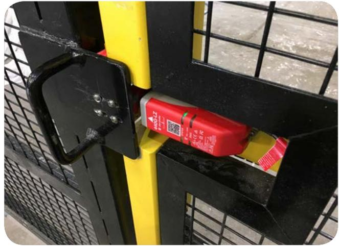
Guardmaster solenoid locking switches used for protection of personnel and machine.
