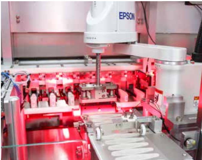
Once filled, the chambers have a plastic film applied and heat sealed using a servo actuator
