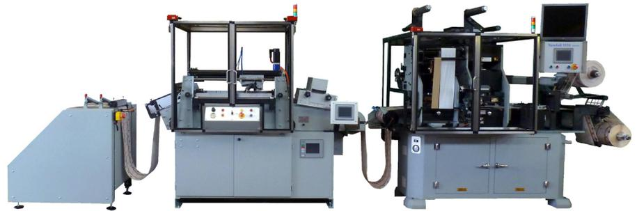
The Servo range comprises seven machine variants, with web widths varying from 175 up to 340 mm
