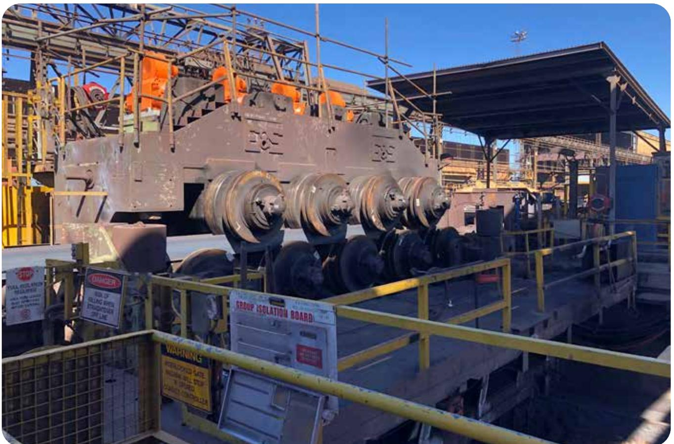
The E&S Straightener machine straightens steel bars of various diameters
