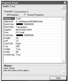
3. To view and edit the tag connection properties for the selected object, select the Connections tab.
