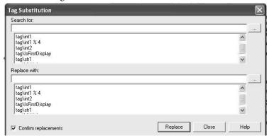
You can use tag substitution on a display-by-display basis to verify that all tags or partial strings are updated correctly in the application.
