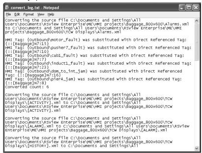
In addition to the conversion log file, the tag converter wizard generates a tag cross-reference .csv file in the destination folder. This file cross-references HMI tags to alias and direct reference tags.
