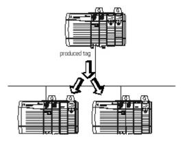
Because a controller produces (transmits) and consumes (receives) data asynchronous to the execution of its control program, the program may begin processing with a mixture of old and new data. Event tasks provide an easy way synchronize the data exchange to ensure that a consuming controller receives all of the data before processing begins.
