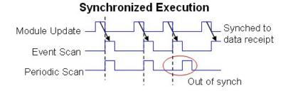
Because each analog module has its own internal sample period for converting analog input signals to digital floating values, an asynchronous loop can exist between the receipt of new input values and the execution of the code for the loop. This discrepancy means that PID calculations execute with stale data, which could result in calculation errors. With an event task, you can easily synchronize the PID calculation to the arrival of flow transmitter data and avoid this potential error.
