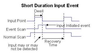
Once the module's Change-Of-State detection captures the input, the module sends this information to the controller. The controller responds and executes the event task even though the input may have turned back off by the time the code in the event task executes.
