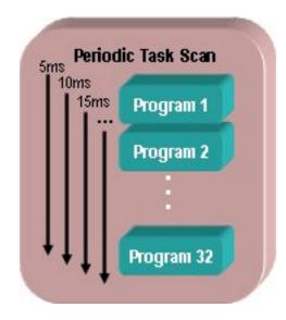
Because you can have multiple periodic tasks that can be triggered at the same time, the controller needs to determine which tasks it can or cannot interrupt. This is accomplished by way of a priority setting for each period task.
