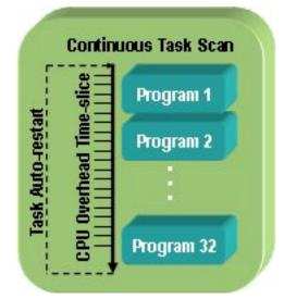
In a Logix5000 controller, the continuous task operates as a background task at the lowest priority. It uses any CPU time that remains after the controller executes the other tasks.
