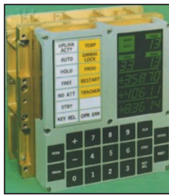
Photo: The Display and Keyboard unit, or DSKY, the interface for the Apollo computers
