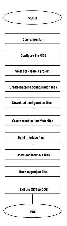
This figure shows a flowchart of the typical ODS process.
