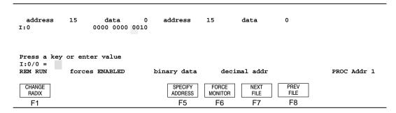
The display area shows input word I:0. Bit I:0/1, the address of the instruction you forced, is set (1). The input data file reflects installed *and* enabled input forces.
