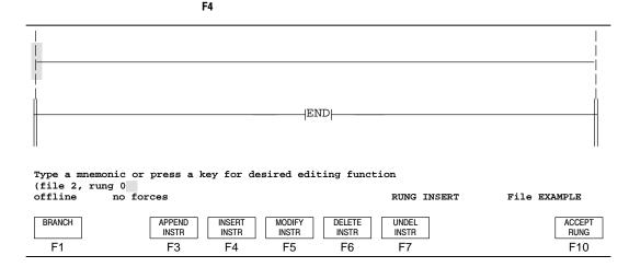
An empty rung appears. The power rails of the rung are broken lines, indicating that the rung is not yet accepted. The cursor is on the left power rail of the rung. The data entry line indicates this to be rung 0. (The end rung is now rung 1.) The status line indicates RUNG INSERT, the current function.
