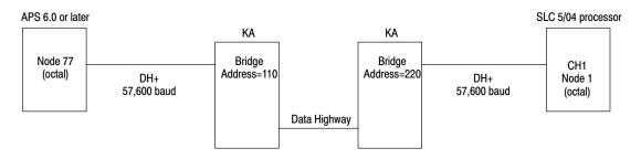
ONLINE CONFIGURATION -Current Device 1784-KT (DH+ Bridged) F1 Bridge Type DH+ to DH+ via two 1785 KA Terminal Name Terminal Address 77 (octal) Baud Rate 57600 F5 SLC Node Address 1 (octal) 110 (octal) F6 Local Bridge Address F7 Remote Bridge Address 220 (octal) IRQ Board/Memory Address 001011 F8 Curr. Interchange Port 1 F9 Save to File ESC exits/Alt-U aborts changes ·
