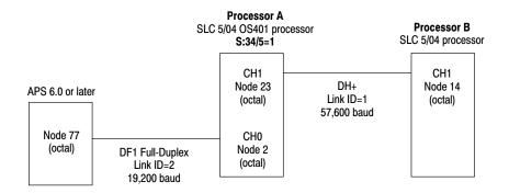
To program the SLC 5/04 OS401 processors on DH+, use the DF1 full-duplex driver. As shown in the screens that follow, enter the destination address 19 decimal for processor A, and enter the destination address 12 decimal for processor B.
