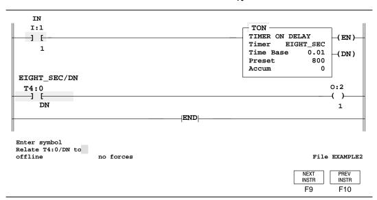
5. EIGHT\_SEC appears within the TON instruction and also above the XIC instruction associated with the timer instruction. Note that the Done bit in rung 1 was automatically assigned the symbol EIGHT\_SEC/DN. If you choose, you can assign a different symbol for the Done bit. For example, type: eight and
