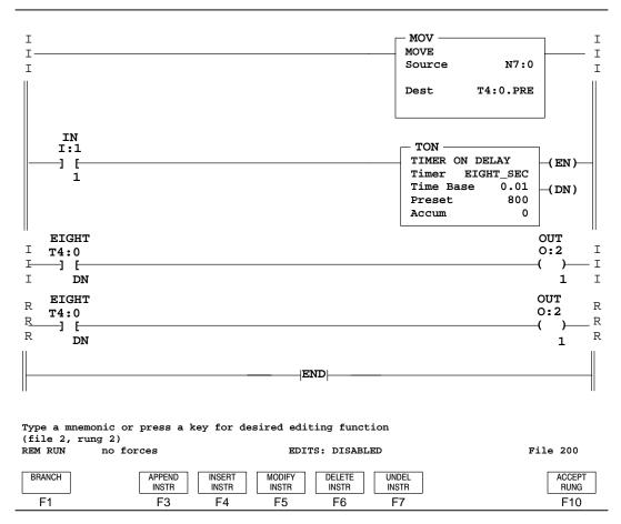
5. Select BRANCH and add a branch to the output instruction. After entering the F1 address, the following display appears:
