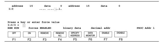
A period indicates that no force is installed. A 0 indicates that a force OFF is installed. A 1 indicates that a force ON is installed. The status line indicates whether the installed forces are enabled or disabled.
