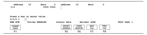
The output data file indicates that O:0/0 is false. The data file bit is unaffected by the forced output.
