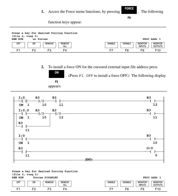
ON appears with instruction I:0/1 in rungs 0, 1, and 2. The status line indicates forces DISABLED. The controller's Forced I/O LED is flashing.
