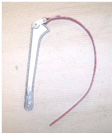
Figure 2.6 – Typical Strap Wrench (not supplied) used to tighten unions on CPVC pipe splices
