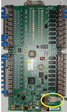
XIO link cable connected to XIO link A
