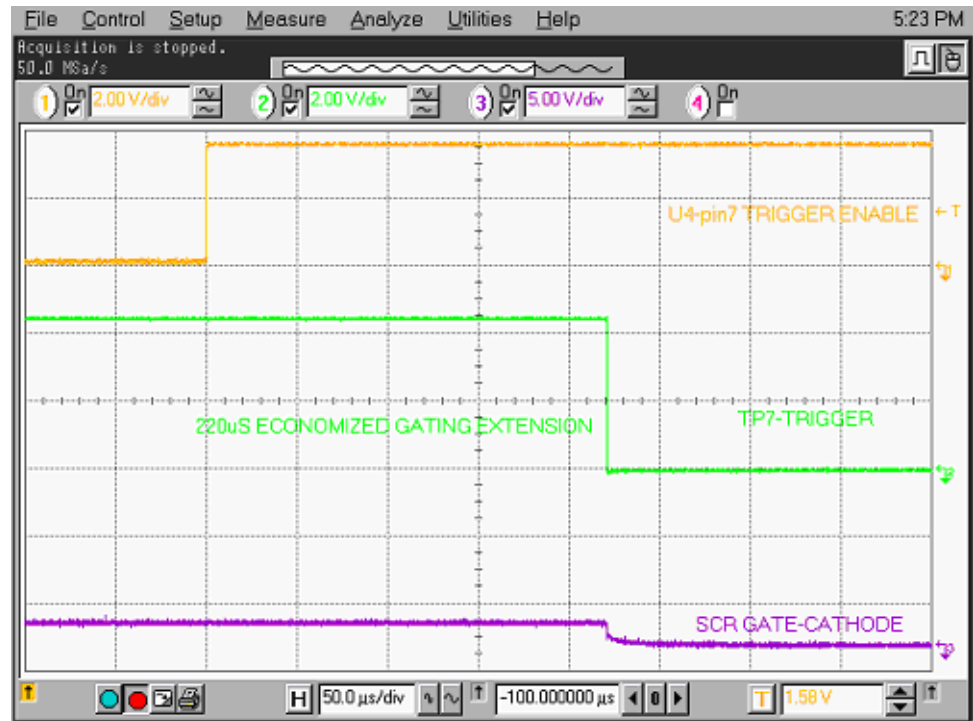
Figure 66 - Expansion of V Sense Trigger to SCR Gating Pulse
