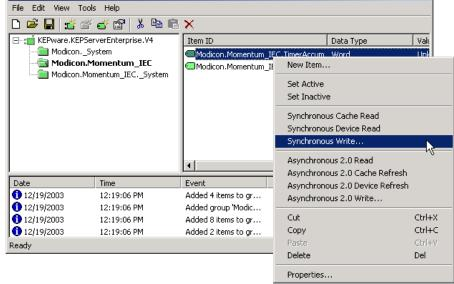
The resulting window not only allows you to write new data to the controller, but it also displays the current value of the tag.
