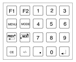
The MicroView uses a sealed membrane, tactile feedback keypad. The keys are color coded to easily identify key functions.
