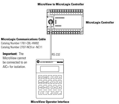
Programming the MicroView The MicroView is programmed off-line using a personal computer running MicroView Programming Software (MDPS). Operating system upgrades can also be transferred using an  $\text{IBM}^{\text{TM}}$  compatible personal computer.
