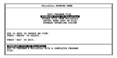
**9.** Highlight "Download File to MicroView" and press [Return]. The Communication Port Selection screen appears. You will not see this screen if a communication port was specified during DPS installation.
