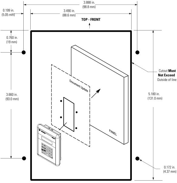
**4.** Alternately tighten the mounting nuts until the terminal is held firmly against the panel. Tighten mounting nuts to a torque of 10 inch-pounds. Do not over-tighten nuts.
