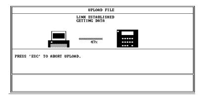
**Note:** If a communication link does not occur in 60 seconds, you get an error message. Check cable connections and verify that the MicroView is in the Program Mode.
