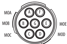
Figure 38 - Monitor Connector Pinout (P2)
