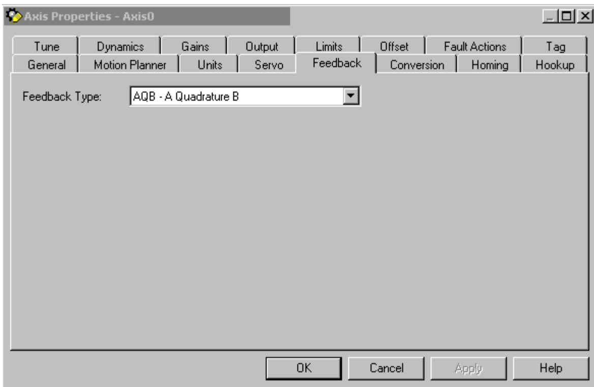
Figure 6.12 Axis Properties - Feedback Tab for Axis_Servo
