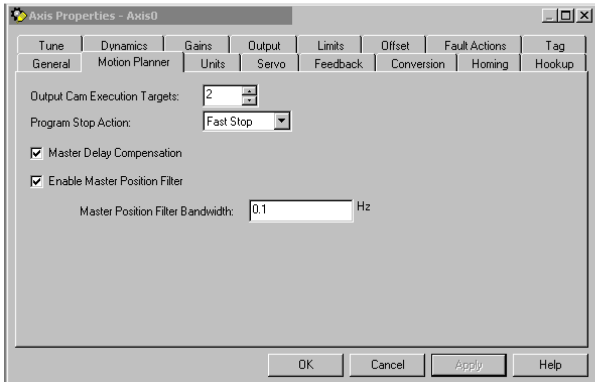
Figure 6.9 Axis Properties – Motion Planner Tab
