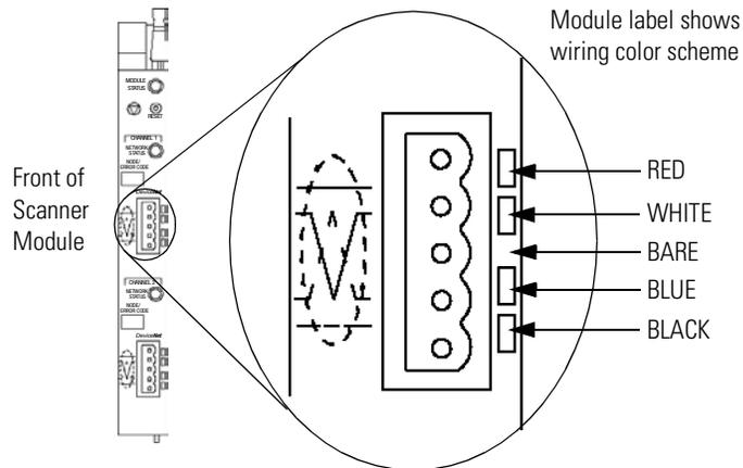
2. Locate the DeviceNet port connector for Channel 1 on the front of the module.
