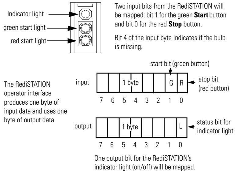
In the RediSTATION's bits for the red and green buttons and the indicator light status bit:
