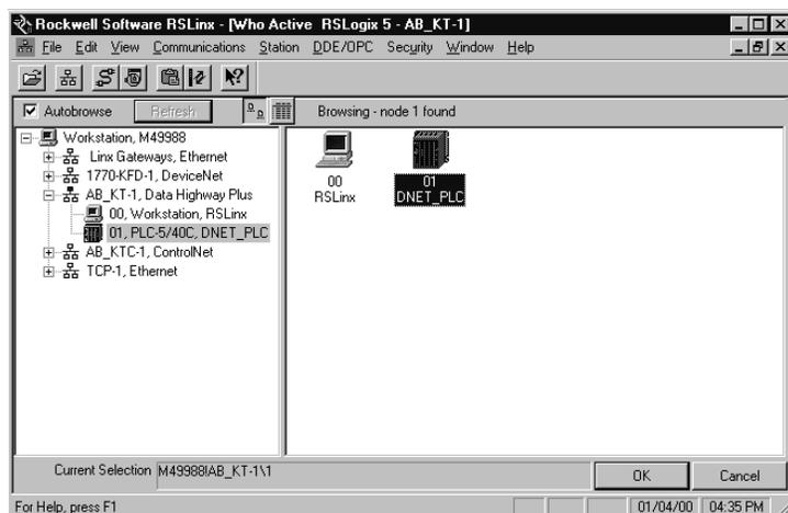
3. Expand the tree under your DH+ driver and highlight the PLC-5 processor as shown above. Click on **OK**.
