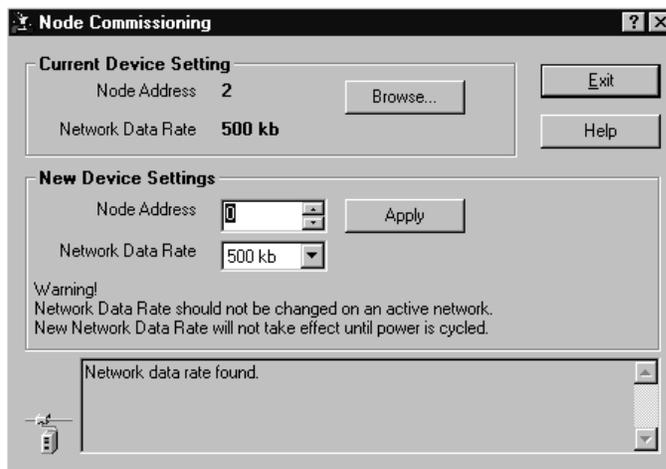
5. In the **New Device Settings: Node Address** box, enter the new node address (e.g., a **0** as shown above).
