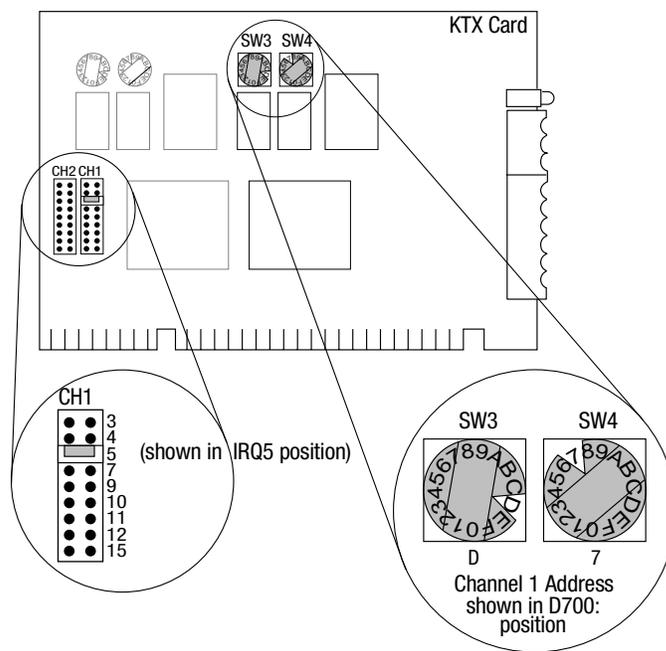
1. Set the interrupt jumpers on the communication card (IRQ5 in this example).
