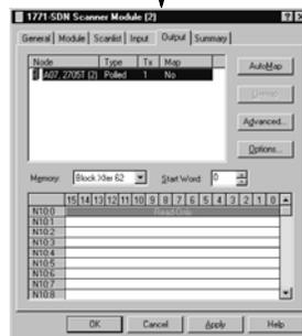
To edit a device's I/O parameters, double-click on the device in the scanlist.
