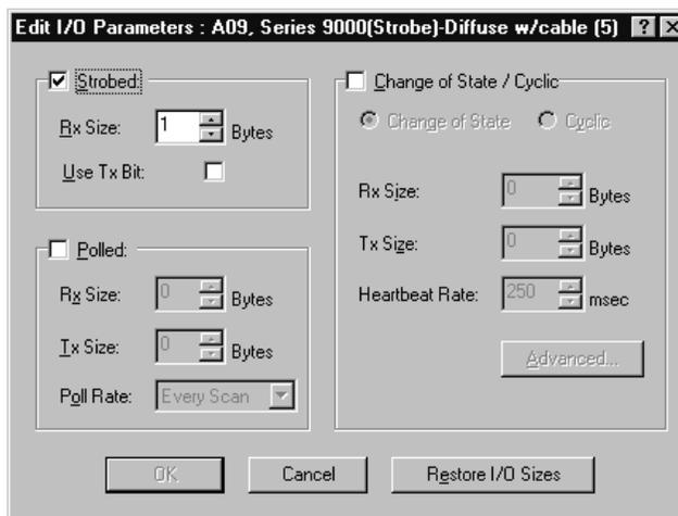
The I/O parameters define the configuration for the device in terms of how much and what data the device will exchange with the 1771-SDN module. By default, the photoeye will send 1 byte when it receives a strobe request. Recall from chapter 3 that the output of the photoeye will be returned in bit 0 of that byte.
