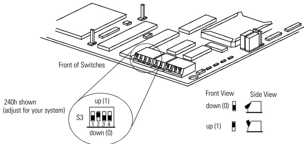
These settings depend on the devices installed on your computer. We used the following addresses:
