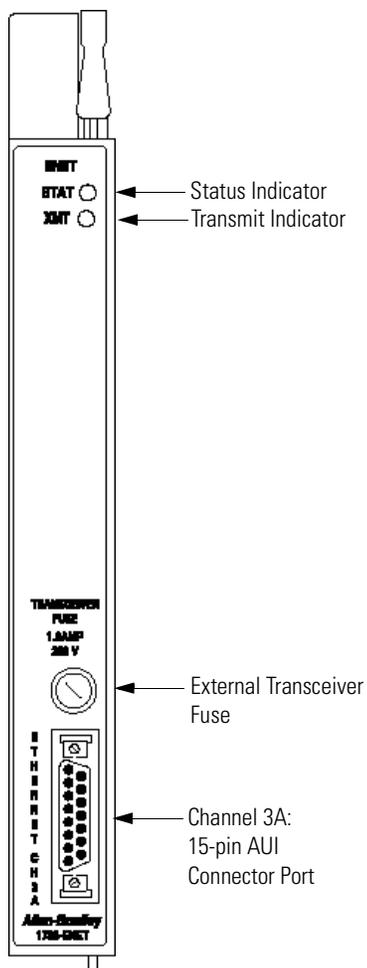
To go online to the PLC-5 processor via Ethernet, you must install a 1785-ENET module in the 1771 I/O chassis.
