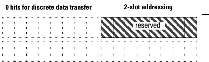
In 2-slot addressing mode, the only memory that would have been available for discrete data transfer (8 bits) is taken up by scanner/processor communication.
