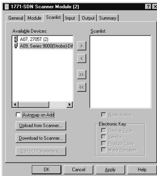
6. For this example, uncheck the **Automap on Add** box, as shown above. You will do this mapping later.
