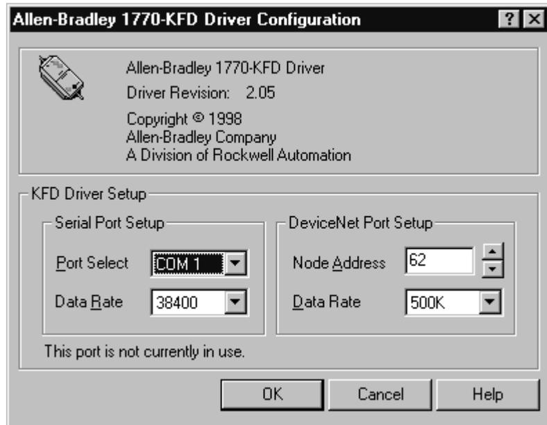
Your driver setup will vary according to your system setup (COM port, Data Rate, Node Address). Choose the appropriate settings for your system. We set the DeviceNet Port Setup Data Rate to 500K for the example application.
