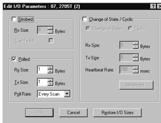
2. Make sure that the **Polled** box is checked and that the **Rx Size** and **Tx Size** are each 1 byte.
