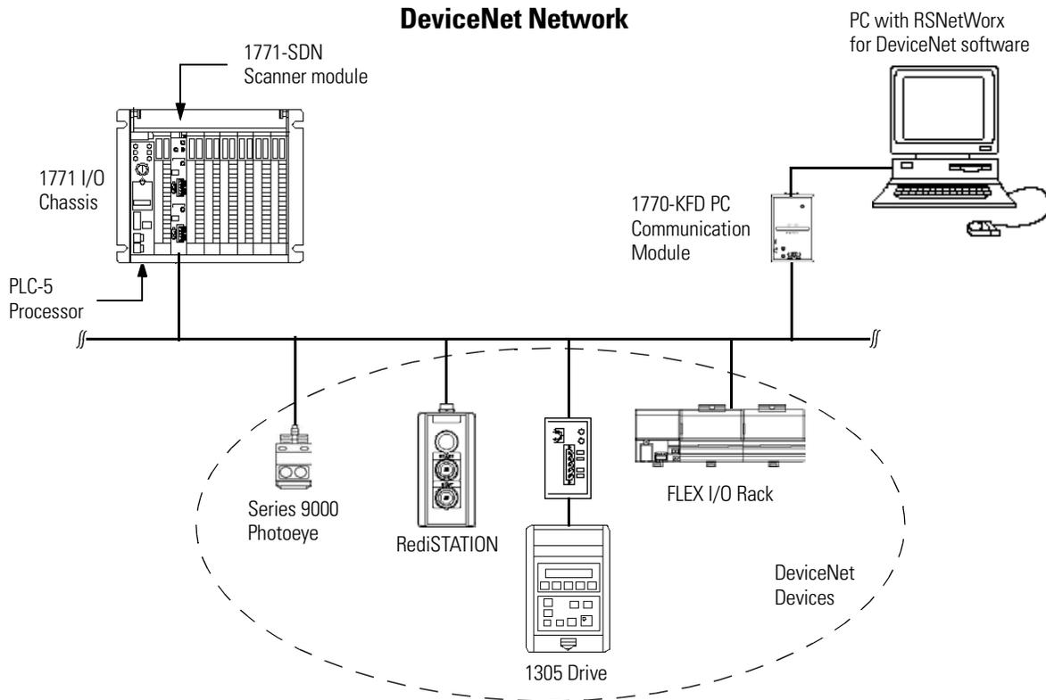
The 1771-SDN module communicates with DeviceNet devices over the network to:
