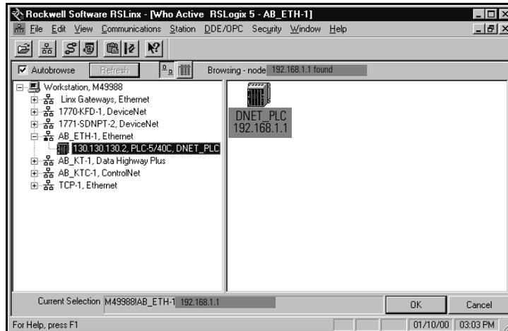
3. Expand the tree under your Ethernet driver and highlight the PLC-5 processor as shown above. Click on **OK**.
