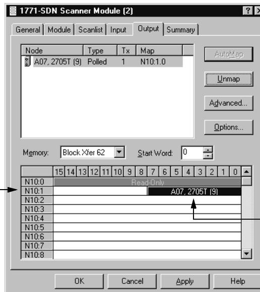
**Note:** The destination address is actually determined by the block transfer instruction in the ladder logic. See chapter 6.
