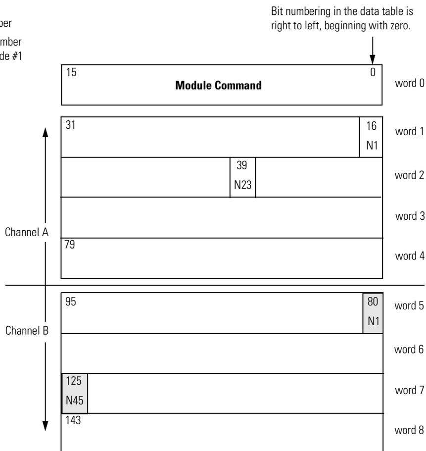
The scanner takes the output bits from its output data table and organizes them into a strobe message. The strobe message contains one bit for each node address, 0-63. In default mode, the scanner is node 63; therefore, this bit is empty. The scanner sends a separate strobe message to each network, via channel A and channel B.
