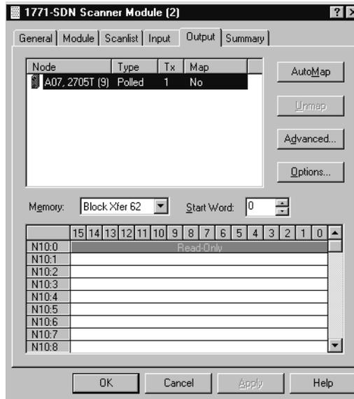
Highlight the RediSTATION as shown above and click on the **AutoMap** button. The mapping of the RediSTATION will appear in the lower panel.
