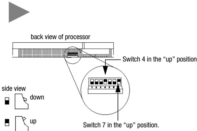
2. Set the baud rate to 57.6 Kbaud by placing switch 7 in the up position.
