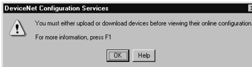
6. Click on **OK** to upload the devices. RSNetWorx for DeviceNet will begin browsing for network devices.
