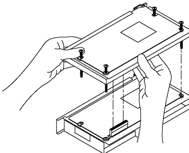
3. Insert the interface module/processor combination in the left-most slot of the 1771 I/O chassis.
