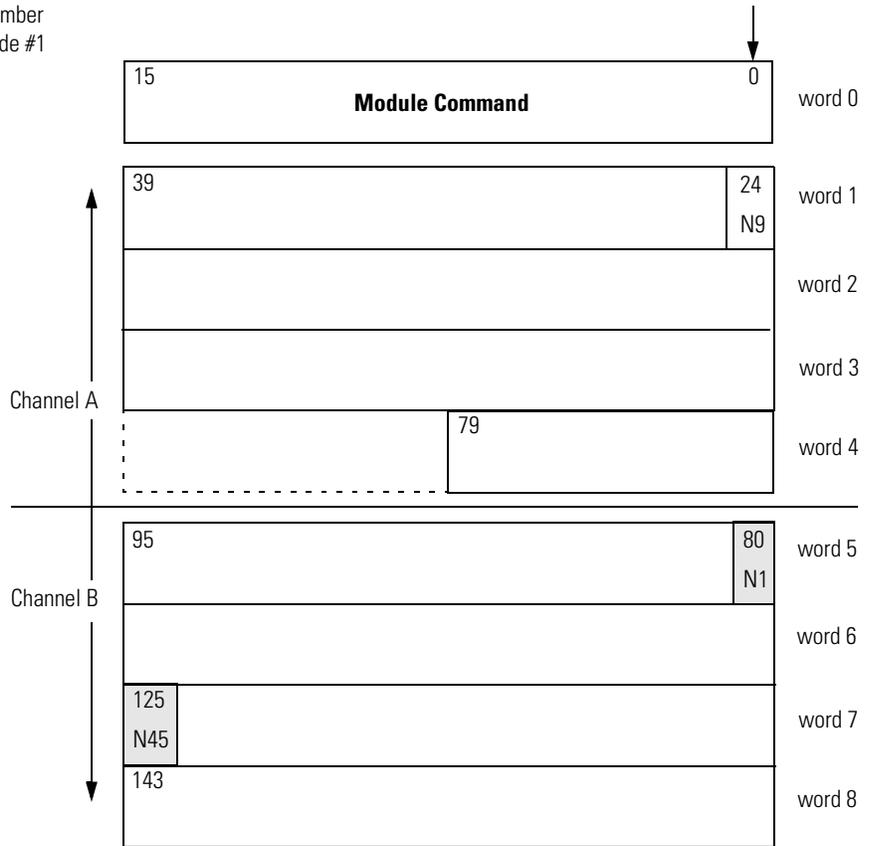
The scanner takes the output bits from its output data table and organizes them into a strobe message. The strobe message contains one bit for each node address, 0-63. In default mode, the scanner is node 0; therefore, this bit is empty. The scanner sends a separate strobe message to each network, via channel A and channel B.
