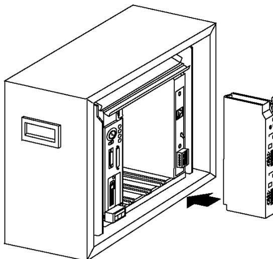
Apply firm, even pressure to seat the module in the I/O chassis backplane connectors.
