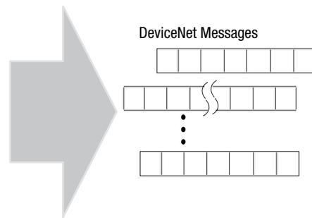
Each individual block transfer is independent, but always retrieves the same input bytes from the scanner's input data table. The types of information that a PLC-5 program will upload from the scanner via the BTR are the:
