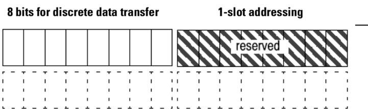
In 1-slot addressing mode, there are 16 bits: eight bits for scanner/processor communication, and eight bits for discrete data transfer.
