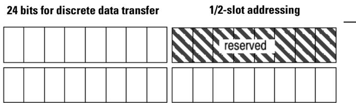
In 1/2-slot addressing mode, there are 32 bits: eight bits used for scanner/processor communication, and 24 bits for discrete data transfer.
