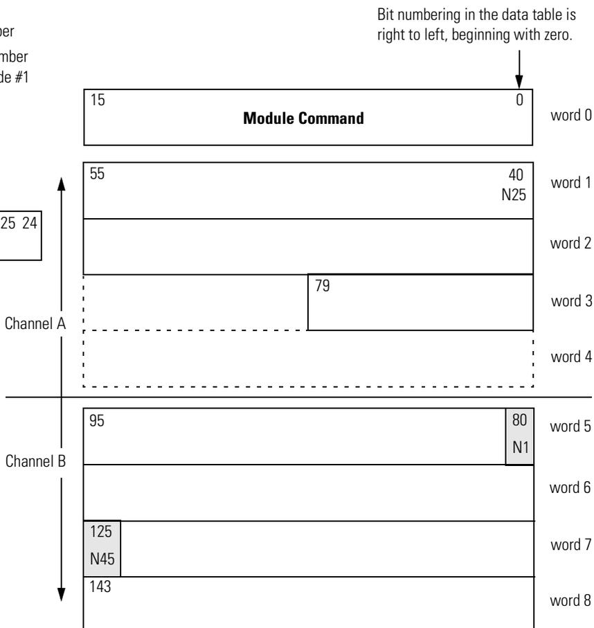
Each node's output bit is mapped to a bit number in the strobe message that directly corresponds to that particular node's MAC ID. For example, the output bit for node #23 is mapped to strobe bit #23.
