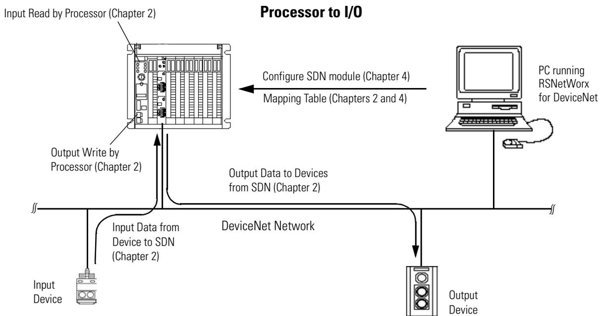
The 1771-SDN scanner module can also be used to bridge a DeviceNet network with another network.
