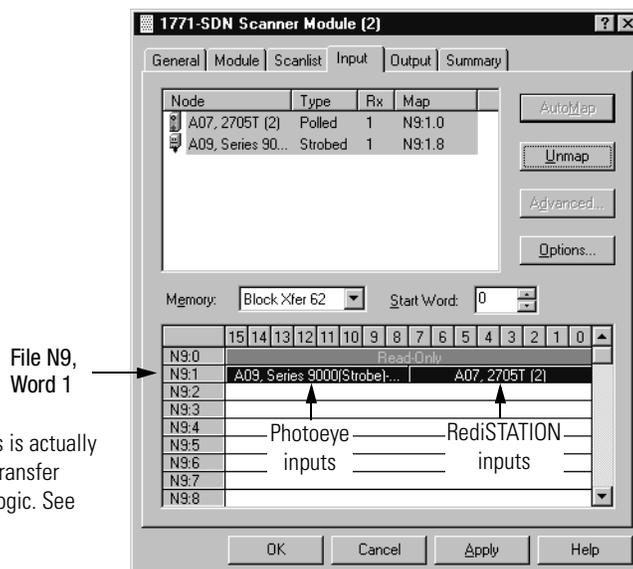
**Note:** The source address is actually determined by the block transfer instruction in the ladder logic. See chapter 6.
