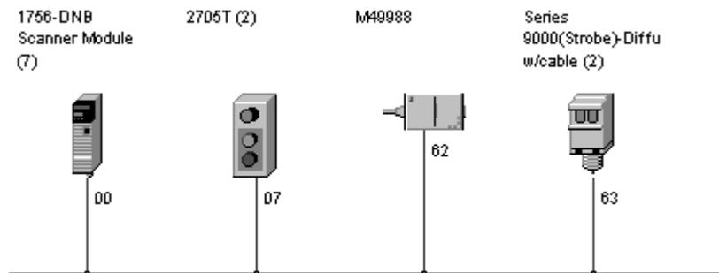
You are now online to the DeviceNet network via the Data Highway Plus network. See pages 4-6 to 4-17 of this manual for examples of how to use RSNetWorx for DeviceNet to adjust network parameters.
