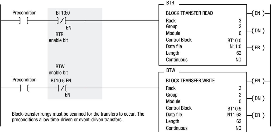
As soon as an asynchronous block transfer completes, it is requested again, independent of other block transfers going to the same module. If you have programmed many block transfers to the same logical rack (especially a remote rack), you will fill the processor’s queue. In this situation, the asynchronous method can result in irregular timing between successive executions of the same block transfer.
