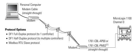
(1) Series C or later cables are required for Class I Div 2 applications.
