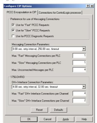
Interval be increased from the default of 1.25 seconds to 8 seconds as shown in the following figure.
