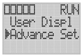
**2.** Then, press the OK key on the LCD keypad. The Advanced Settings Menu screen is displayed, as shown below.
