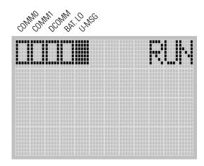
Note that the U-MSG indicator on the top of the LCD is displayed in solid rectangle. It means the LCD is in User Defined LCD mode.
