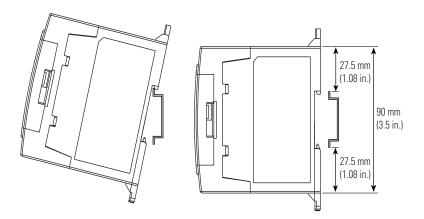
Follow this procedure to install your controller on the DIN rail.
