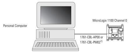
(1) Series C or later cables are required for Class I Div 2 applications.
