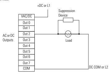
If the outputs are DC, we recommend that you use an 1N4004 diode for surge suppression, as shown below. For inductive DC load devices, a diode is suitable. A 1N4004 diode is acceptable for most applications. A surge
