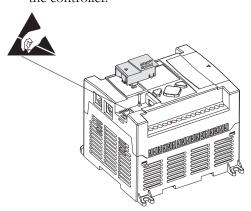
**3.** Firmly seat the memory module into the controller.
