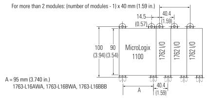
NOTE: All dimensions are in mm (inches). Hole spacing tolerance:  $\pm 0.4$  mm (0.016 in.).
