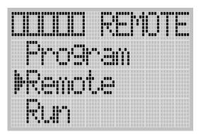
All the built-in LCD screens except the Boot Message screen display *the current mode switch position*, at their top right portion, as shown below. In this example, the mode switch position is set to RUN.
