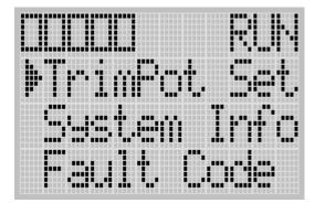
**2.** Then, press the OK key on the LCD keypad. The Trim Pot Select screen is displayed, as shown below.
