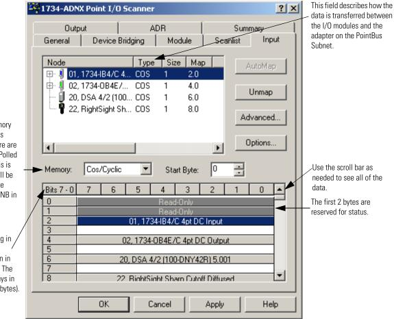
Scroll down and notice that bytes 0 through 8 = 9 bytes total were enough for the input data.
