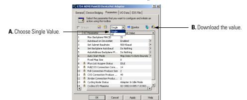
After 30-40 seconds, the adapter begins operations and uses the configuration most recently applied. During the auto start mode process, the Physical List Acquire Status field displays the words: *Auto Start Mode*, but after the download is complete the field displays the word: *Idle*.
