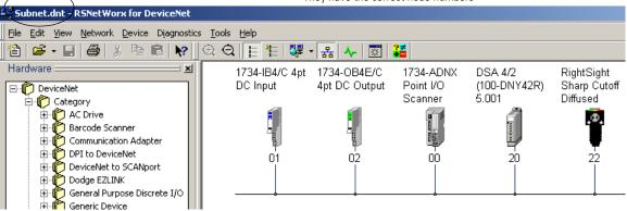
On the Subnet, the 1734-ADNX is a scanner and it is always at node 0. It is OK for some or all of the node numbers on the Subnet to be the same as devices on the primary network. Because they are two different networks, duplicate node errors will not occur. The 1734-ADNX will communicate back to the 1756-DNB scanner as a single entity (only taking up one node number on the main network).
