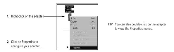
You see a pop-up screen with a series of tabs. Each tab provides options to write configuration for your adapter. The tabs are shown below and on the following pages.
