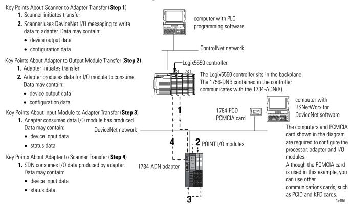
Because the adapter simultaneously resides on the DeviceNet network and on PointBus, it serves as a slave to the processor (i.e., #1 & 4) and a master to the I/O modules (i.e., #2 & 3).
