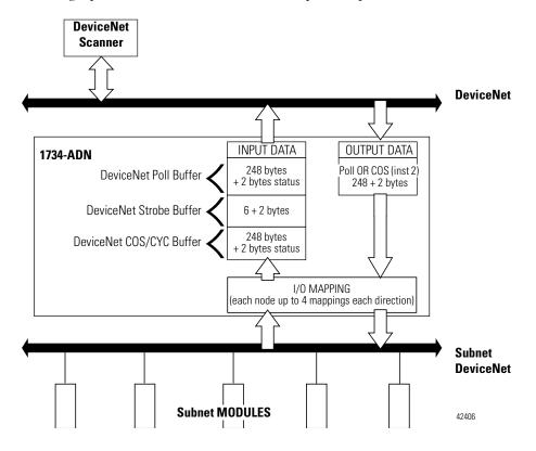
See Table 2.A for definitions of the first 2 bytes of each I/O message produced by the adapter on DeviceNet.
