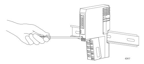
**5.** Pull the adapter off of the DIN rail to remove it from the existing system.
