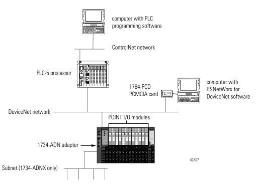
After you have installed your adapter into a POINT I/O system, you must perform the following tasks:
