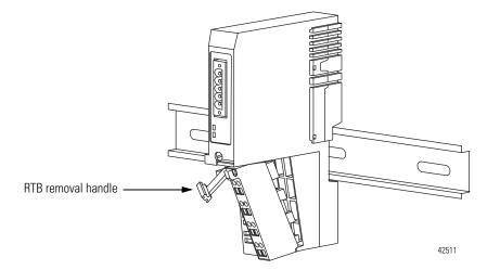
**4.** Use a small bladed screwdriver to rotate the DIN rail locking screw to a vertical position and release the locking mechanism.
