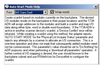
Right now, the 1734-ADNX is not in another scanner's scanlist so you can use the Auto Start Mode feature. By using Auto Start Mode, the 1734-ADNX will map all the devices on the Subnet and automatically adjust the value for parameters 1, 9, 10, 11, and 12.
