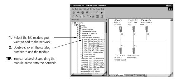
You must configure the modules connected to the scanner. For more information on how to configure POINT I/O modules, see the POINT I/O Digital and Analog Modules and POINTBlock I/O Modules user manual, publication 1734-UM001.
