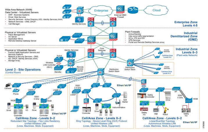
Multiple Cell/Area Zones, each containing different types of connectivity topologies, reside at the edge of the IACS application and overall CPwE architecture. The lightly managed IES that are highlighted by a green rectangle representing where a lightly managed IES could be placed. As discussed in Cell/Area Zone, page 1-5, several different supported topologies exist for connecting these lightly managed IES to the rest of the plant-wide network.
