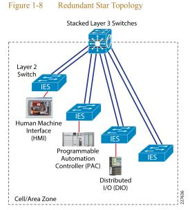
A star topology without redundant links between the IES is also possible, and can help minimize the number of ports and cables required, at the expense of resiliency in the event of an uplink failure. This topology will still help minimize the number of hops required and bottlenecks that exist in some other topologies.
