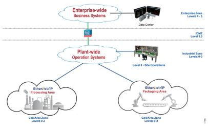
Zooming in on the Industrial Zone (Levels 0-3) shows how a Cell/Area Zone (packaging) can in fact be sub-divided into multiple sub-zones (for example, Lines 1, 2 and 3), as shown in Figure 1-4, and then into further sub-zones for each function within each line (for example, labeling, filling and packaging).
