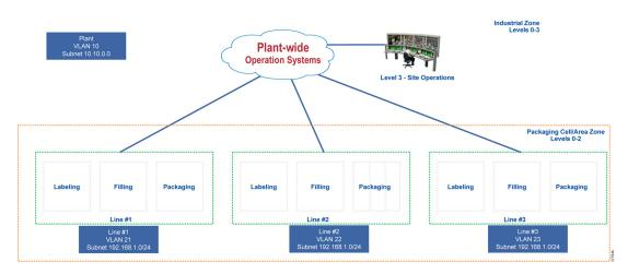
Figure 1-5 zooms further into the individual sub-zones for each packaging line. Zones and sub-zones allows plant operators to achieve scalability through a building block approach. A machine or skid are examples of how these sub-zones could be used.
