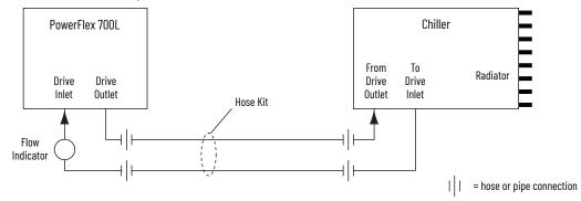
The drawing below shows a cooling loop diagram for a typical chiller.
