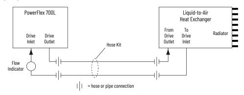
The drawing below shows a cooling loop diagram for a typical liquid-to-air heat exchanger.
