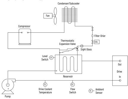
The main components of the chiller cooling loop are listed below.
