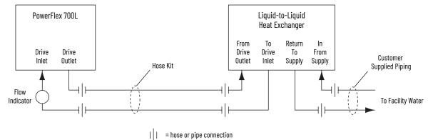
The drawing below shows a cooling loop diagram for a typical liquid-to-liquid heat exchanger.
