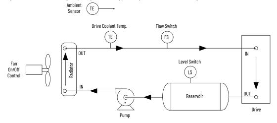
The main components of the liquid-to-air heat exchanger cooling loop are listed below.
