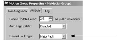
With this revision, a motion group that is configured to produce a major fault produces a major fault *only* if the controller is in run/remote run mode.
