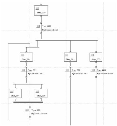
Execution starts at Step\_000. When Tran\_000 becomes true, Step\_001, Step\_002 and Step\_003 should become active. However, because the nested simultaneous branch in the left path converged and looped back to its parent step (Step\_001), the active steps were actually **Step\_005**, Step\_002 and Step\_003.
