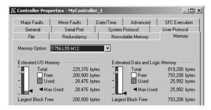
When online with a controller, the *Memory* tab shows the actual memory usage of the controller. The tab includes a *Max Used* entry for each type of memory. The *Max Used* values show the peak of memory usage as communications occur.
