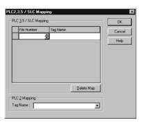
A Logix 5000<sup>™</sup> controller stores tag names on the controller so that other devices can read or write data without having to know physical memory locations. Many products only understand PLC/SLC data tables, so the Logix 5000 controller offers a PLC/SLC mapping function that lets you map Logix tag names to memory locations.
