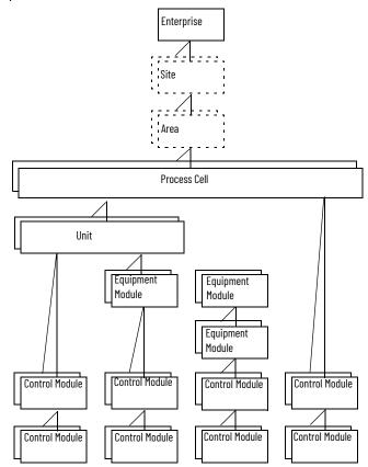
The physical model defines the automation components within a given environment, and determines modular areas and component interactions.
