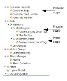
Data scope defines where you can access tags. Controller-scoped tags and parameters are accessible by all programs. Local tags are accessible only by the code within a specific program. Equipment Phases, like Programs, have parameters and local tags.
