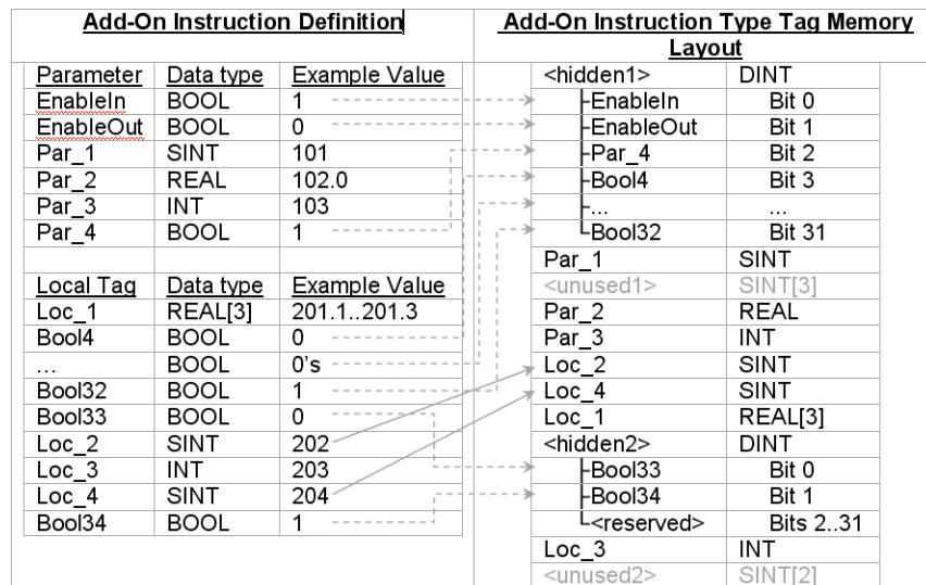
The L5K representation of an Add-On Instruction type tag containing the example values is: [-2147483643, 101, 102.0, 103, 202, 204, [201.1, 201.2, 201.3], 2, 203].
