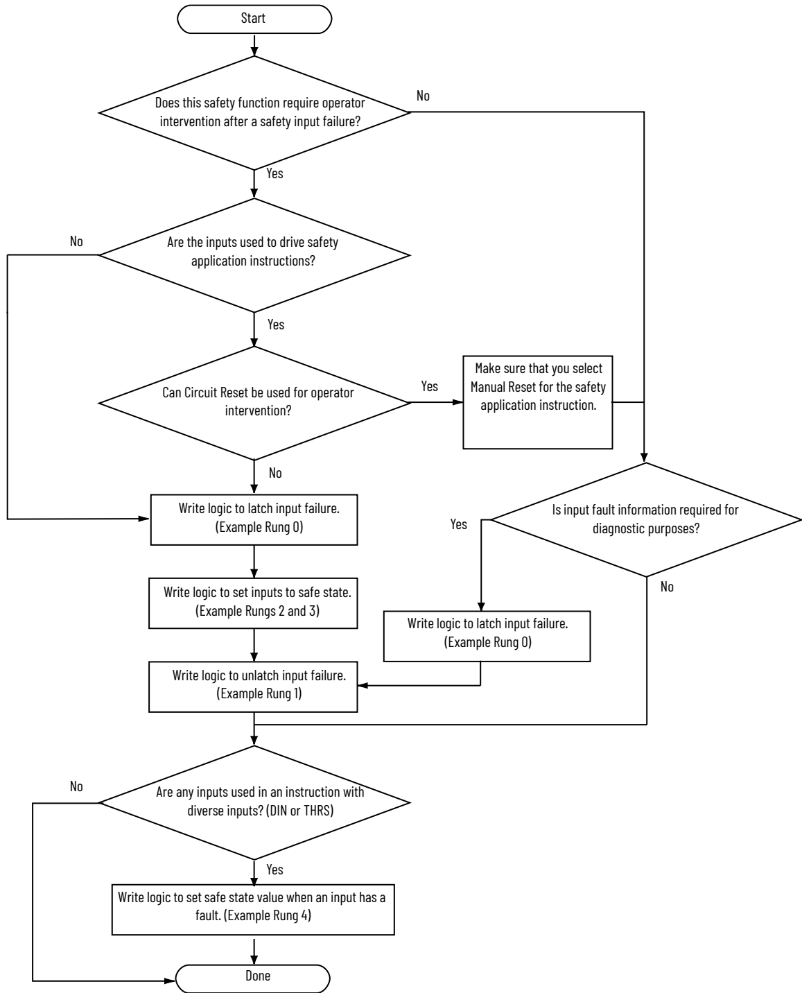
Figure 56 - Input Fault Latch and Reset Flowchart
