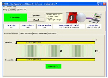
This screen lets you monitor the status of the light curtain when a computer is attached to the MSR42 relay via the Optical Interface. It has other helpful diagnostic features which are described in the MSR42 Safety Base Module Operation Manual, publication 440R-IN017, and the Configuration Tool for MSR42, GS Micro400 and Safe 2/4 Light Curtains Software Description document, available on the CD that ships with the Optical Interface tool.
