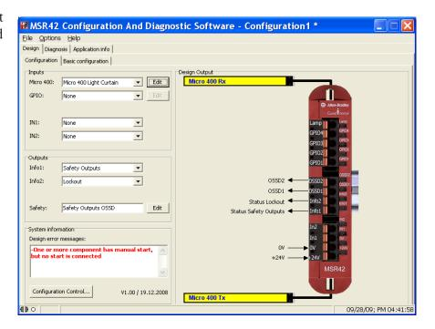
**4.** On the Configuration dialog box, select Start from the IN1 Inputs pull-down menu.
