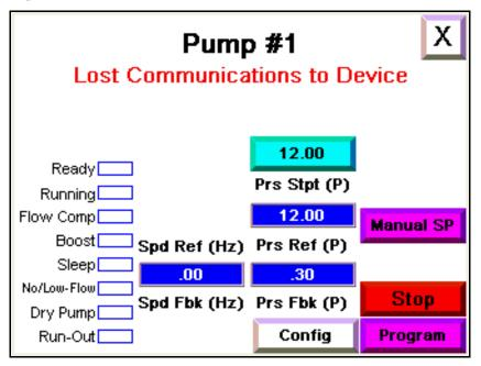
**2.** Plug the RJ45 connector back into the drive. The Lost Communications to Device message disappears and the F81 Comm Loss fault displays.
