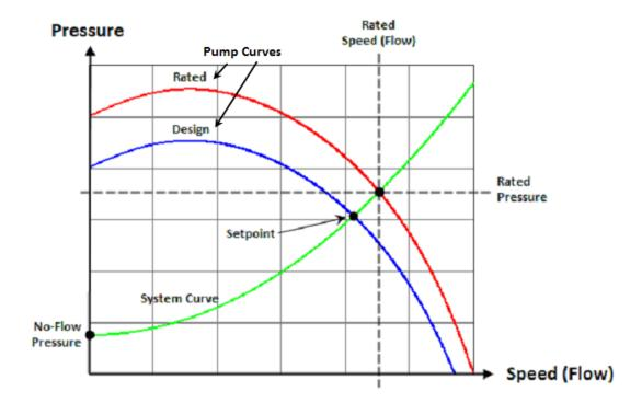
To achieve the best results, the calculated system curve needs to precisely match the actual system curve. This can be accomplished by adjusting the curve approximation. A curve approximation of 0%, will produce a linear result and may reside above the actual curve.
