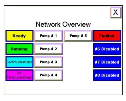
Since you have already verified that communication between the MicroLogix controller and the PowerFlex 400 drive(s) is working, once the PVc application is running, any drives that are enabled should be displayed as being 'Ready' on the Network Overview screen.
