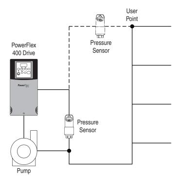
To counteract this over pressure condition, flow compensation reduces the pressure setpoint according to pump speed (which is approximately proportional to flow) to help maintain a constant pressure at the user point.
