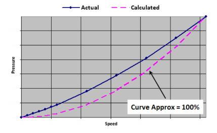
Determining the best curve approximation may require quantitative knowledge of the actual system curve. Please reference the Flow Compensation System Curve Calculator.xls (located on the Connected Components Building Blocks Overview DVD, CC-QR001) for a suggested procedure and tool to help determine the optimum curve approximation.
