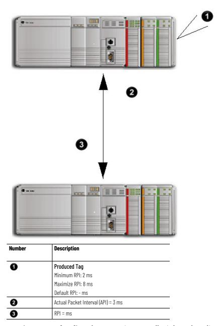
**Version 17.00 and earlier:** The consuming controller is brought online with an RPI configured at 3 ms. The producer accepts the RPI requested by the consuming tag. All controllers on the multicast connection increase to 3 ms for the API, which is the interval the data is actually being produced.
