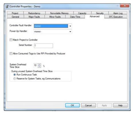
3. Select the Allow Consumed Tags to Use RPI Provided by Producer check box to allow for the RPI negotiation.
