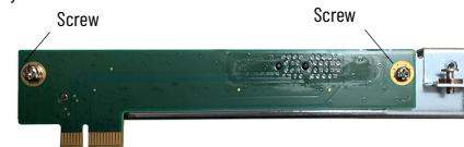
5. Connect the replacement PCI riser card to the add-in card tray with the two screws retained in step 4.
