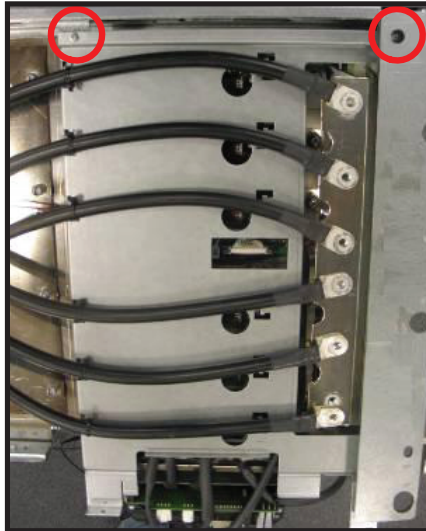
Figure 15 - Removing EMC Shield Cover Screws
