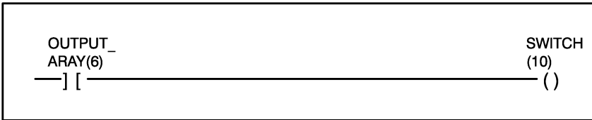
Figure 3.3 - Arrays Used As Contact and Coil
