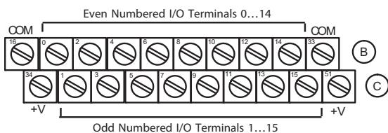
Connect -V (Supply Common) to terminal B-16
