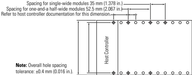
Locate holes every 17.5 mm (0.689 in.) to allow for a mix of single-wide and one-and-a-half-wide modules (e.g. 1769-OA16).
