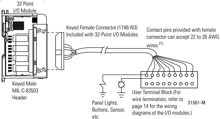
(1) Maximum user cable length is dependent on how much voltage drop (current x ohms/ft.) x (feet) the user's system can tolerate. The user's system should take into account the minimum turn-on voltage required by external loads connected to the 32-point output module, the minimum turn-on voltage required by the 32-point input module, and all of the voltage drops associated with wiring to and from the load, sensors, terminal blocks, power sources and the module itself.
