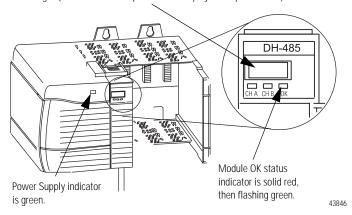
At powerup the module's alphanumeric display begins a cycle through the following sequences.
