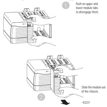
If you are replacing an existing module with an identical one, and you want to resume identical system operation, you must install the new module in the same slot.
