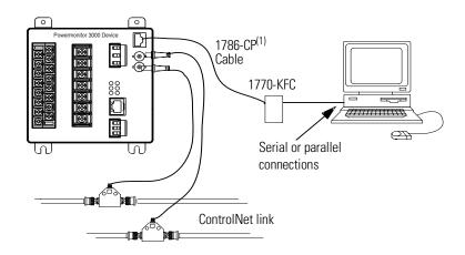
The 1786-CP cable can be plugged into any ControlNet product's NAP to provide programming capability on the ControlNet network. A programming terminal connected through this cable is counted as a node and must have a unique network address.
