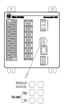
The Powermonitor 3000 is equipped with six bi-color light emitting diodes (LED's) arranged as shown in Figure 5.
