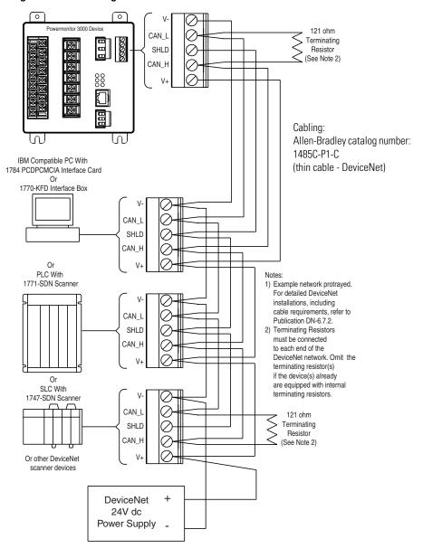
Figure 36 Connecting Powermonitor 3000 to other DeviceNet Devices
