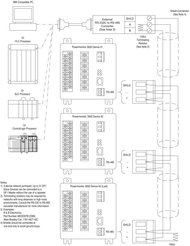
Figure 31 RS-485 Connections
