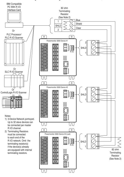
Figure 34 Connecting Powermonitor 3000 to Remote I/O Scanner
