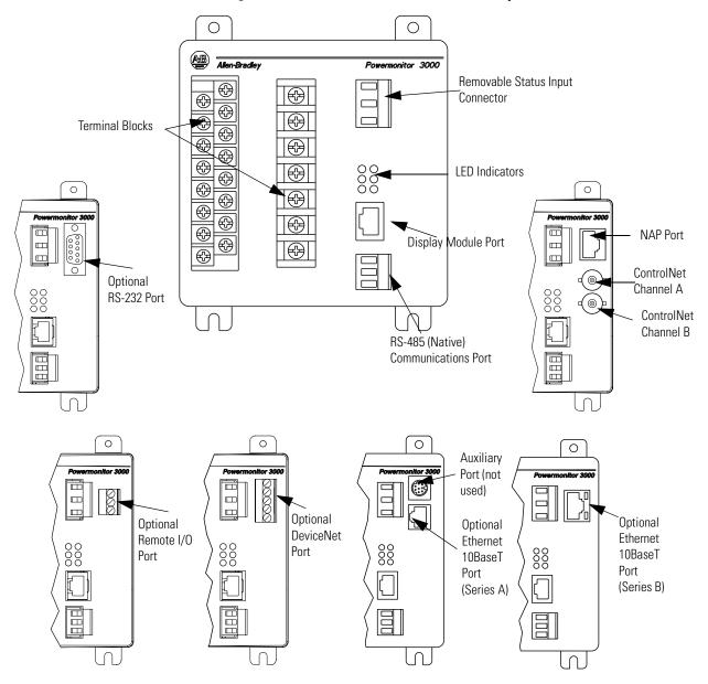
**Figure 3 Master Module with Communication Options**
