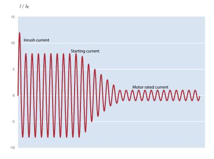
In the picture above, which shows the typical starting phase of an induction motor, three levels of current can be noticed:
