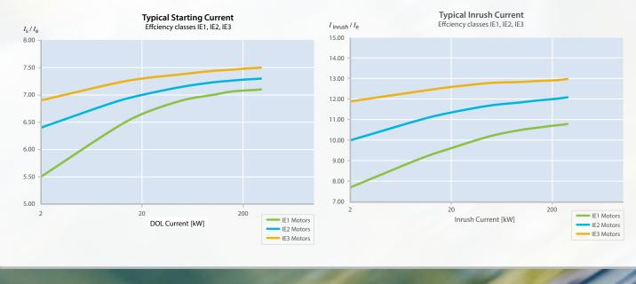
The specific starting current characteristics of the higher efficiency motors are requiring a special attention. A proper selection of the motor starting and switching components will make sure that the application starts without disturbances nor component damages. In particular, the following risks exist and must be avoided:
