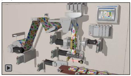
Vertical Form, Fill, and Seal (VFFS) machines are used in the consumer products industry for a wide variety of packaging applications. Various products like salt, tea, sugar, spices, snack foods, wafers, detergent, and candies are placed into formed pouches and then sealed. The pouch material is flexible and typically heat-sealable plastic. Paper is also used and sealed by glue.
