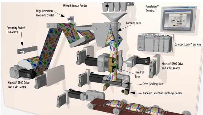
The Rockwell Automation Integrated Architecture™ with Integrated Motion on the EtherNet/IP network is ideal for VFFS machines.
