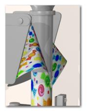
Flat film is converted into a tubular or tunnel shape. The film travels on the outside of the forming tube. The cone and correct diameter tube are combined to form the flat film into a tubular or tunnel-type shape.
