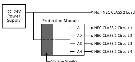
A typical wiring configuration is shown in Figure 2. All sensitive loads are connected directly to the power supply. If needed, these load circuits can be protected with standard circuit breakers or fuses. Loads which are less sensitive to voltage dips or interruptions or which are the source of the voltage drop themselves are connected to the output of the Bulletin 1692 protection module.
