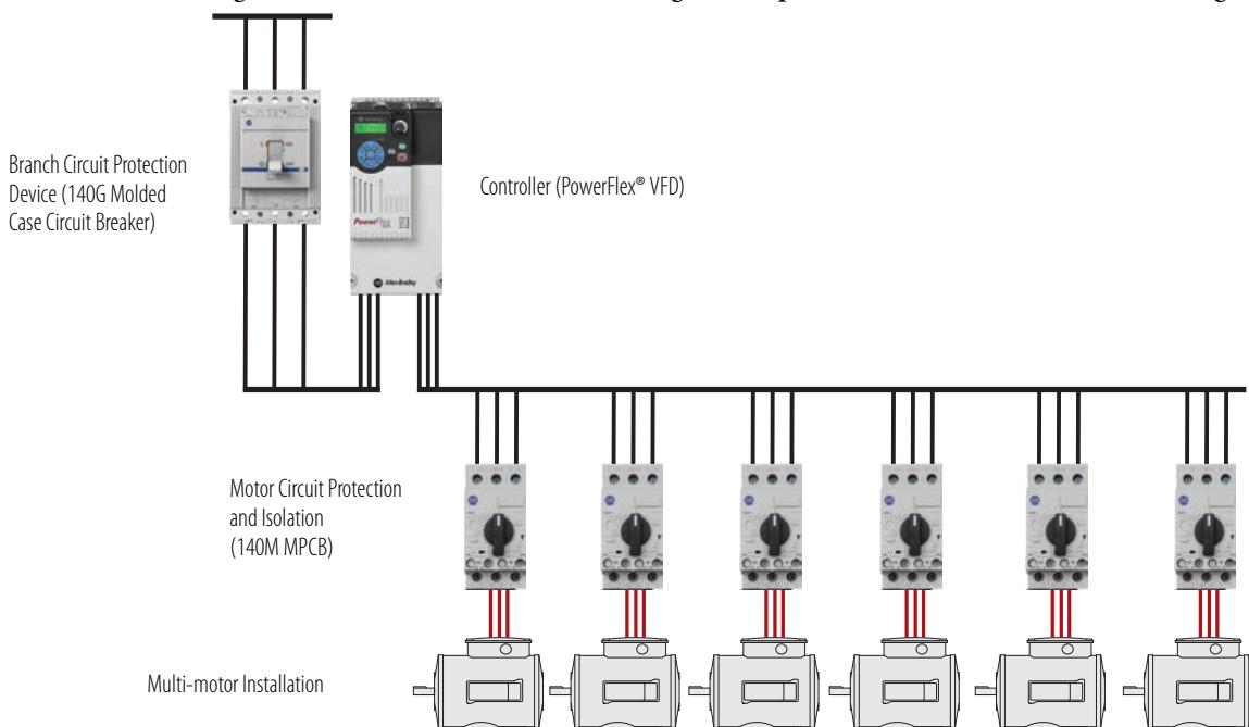
Note: With the PowerFlex 525 Low Voltage Drive, we do not recommend going below 3 Hp in multi-motor applications due to the cable charging current.
