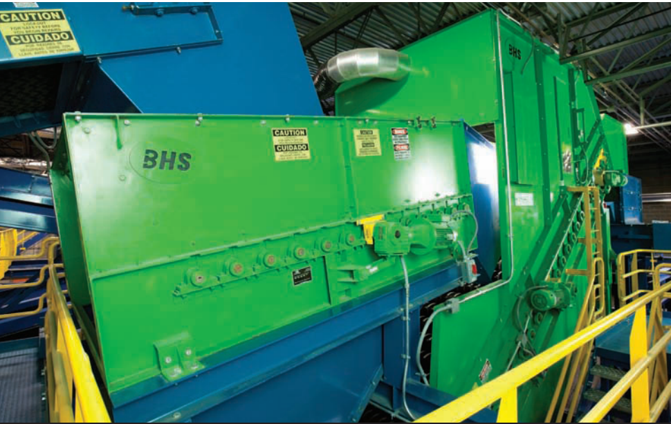
Some of the largest BHS systems are comprised of modular lines handling 50 tons of waste per hour and can be made larger to meet the growing demand.
