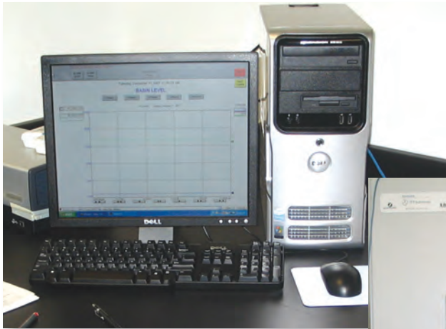
Left: A SCADA system visualizes process data from a plant basin on an operator's desktop PC. Below: ITT-Sanitaire automated the St. Joseph Sanitary District's wastewater treatment plant by installing control panels with CompactLogix PACs. The RSLogix 5000 programming software helped cut installation time in half.
