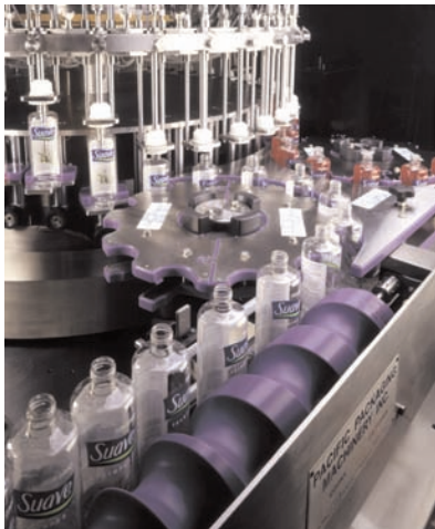
36-Station Rotary Volumetric Filling Machine from Pacific Packaging Machinery
