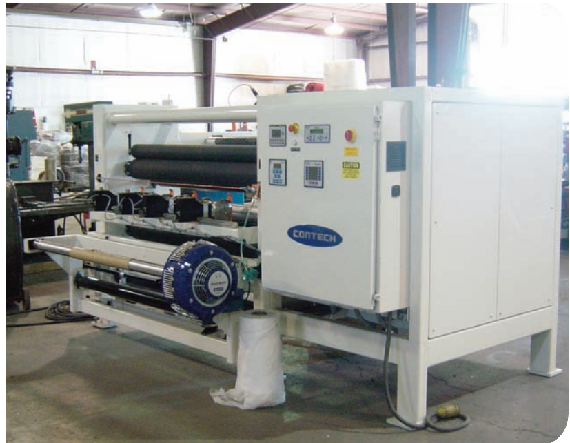
Slitter/rewinder equipment from Contech leverages Connected Component core technologies from Rockwell Automation.
